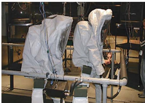
*Fig 4. Evaluation of the heat strain produced in chemical overgarments with Soldier participants exercising on a treadmill in the Doriot climatic chambers. Thermal physiologists at USARIEM have evaluated all chemical pretreatments and personal protective equipment before approval and fielding by the Army.*
